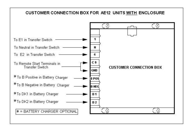
Baldor Generators strongly recommends that all electrical devices share a common ground (i.e. Generator Set, Transfer Switch, Battery Charger, Load Devices, etc.). The grounding stud for the generator set is located under customer connection box.
